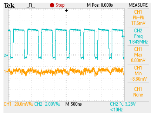
STEADY STATE OPERATION (VIN=5V, VOUT=3.3V, IOUT=1500mA)
