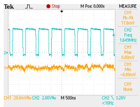
STEADY STATE OPERATION (VIN=5V, VOUT=3.3V, IOUT=1500mA)
