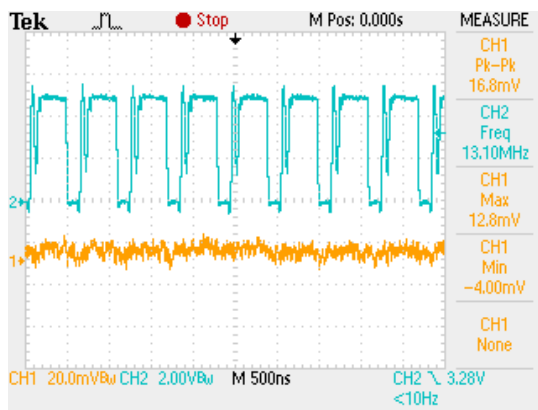
STEADY STATE OPERATION (VIN=5V, VOUT=3.3V, IOUT=100mA)
